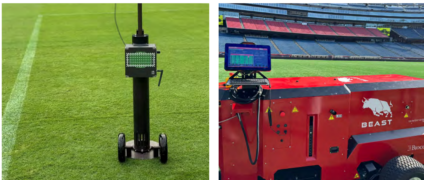
Fig. 60. Biomechanical testing for impact (left) and traction (right)
