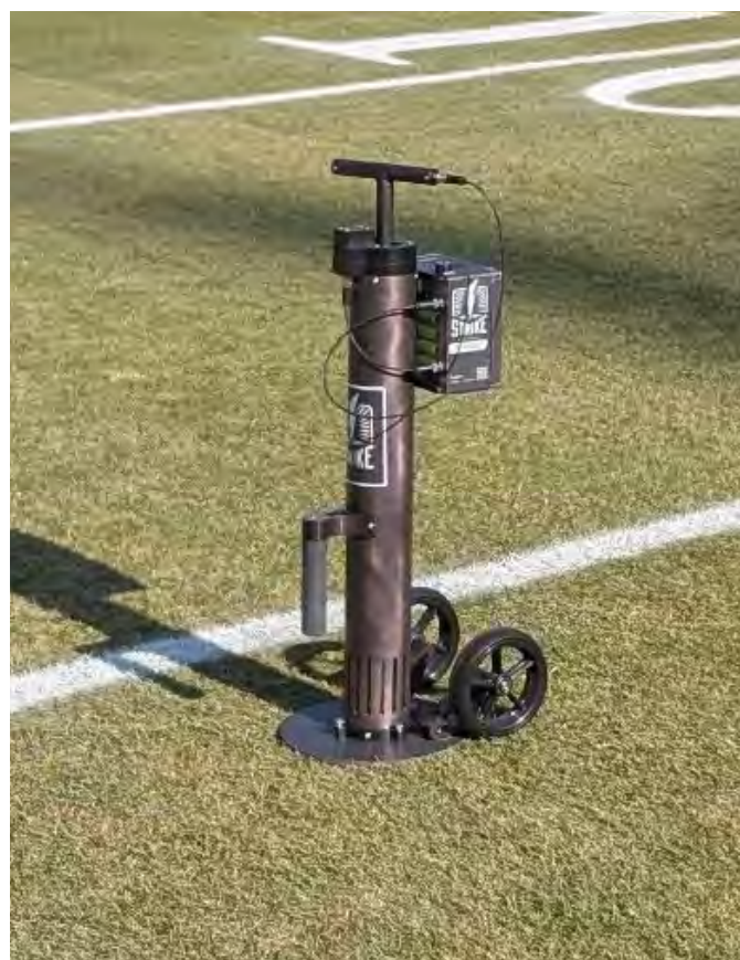
Fig 22. Impact testing on new sod
