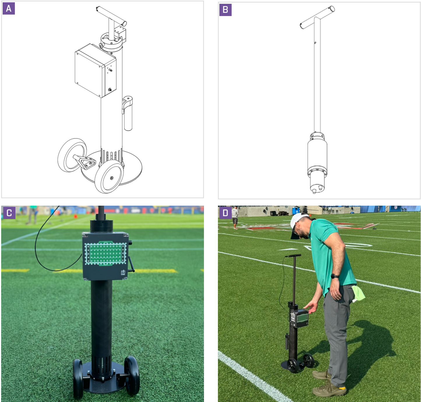
Figure 2. (a) Schematics for the STRIKE device and (b) impact mass; (c) STRIKE in use in a stadium and (d) operator using the STRIKE
